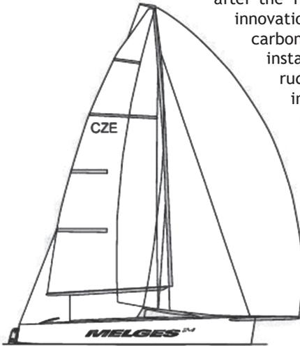
Sailing the Melges 24, simple is the key word here. The boat is very stable with its minimum weight aloft and maximum weight down below. The carbon keel fin weighs just 35 pounds while it supports a lead bulb of 630 pounds five feet below. This makes for a comfortable sail in all conditions. No winches! No winches are needed upwind or downwind on this 24-foot boat. This makes your crew
